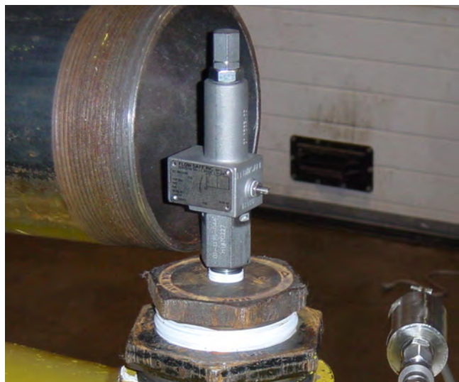
Certification flow test of F84M-1
